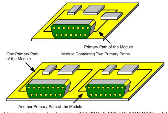
A test connector is an external path whose TAP\_SCAN\_CLOCK, TAP\_SCAN\_MODE, and, if present, TAP\_SCAN\_RESET ports all have mode IN or mode INOUT. Such an external path may be controlled by a test controller. A *unit-under-test connector* is an external path whose TAP\_SCAN\_CLOCK, TAP\_SCAN\_MODE, and, if present, TAP\_SCAN\_RESET ports
