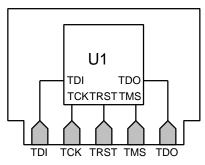
The connector has the five TAP signals (TAP\_SCAN\_IN, TAP\_SCAN\_OUT, TAP\_SCAN\_CLOCK, TAP\_SCAN\_MODE, and TAP\_SCAN\_RESET) each wired appropriately to the member device. What are the important characteristics of this module?
