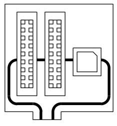
This example board contains two backplane slots, one chip socket, and one card-edge connector, all of which are scannable. No scannable devices or modules are wired onto the board, only connectors for plugging in other things later. From the HSDL point of view, this module appears as shown here.
