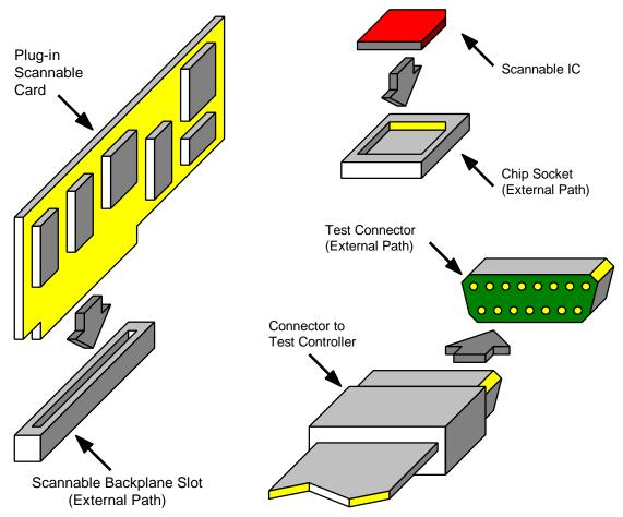
A serial TDI-to-TDO connection of member devices, member modules, and paths that all share the same TAP control signals is a *static path*. A static path represents a simple wiring-
