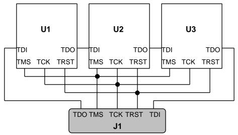
The static path depicted here has four items in it: three devices and one external path. Since an external path describes the ports used to control it, the static path containing the external path completely describes the netlist of the test bus. All connectivity information for TDI, TDO, TMS, TCK, and TRST signals can be derived.
