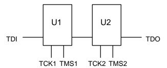
In this module, the connection of devices does not correspond to the HSDL definition of a scan path; that is, serially connected members or paths sharing the **same set of TAP control signals**. These devices are serially connected, but they are connected to different TAP\_SCAN\_CLOCK and TAP\_SCAN\_MODE ports.
