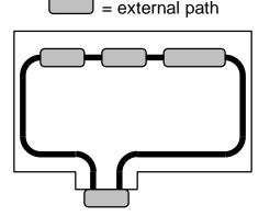
So the module is composed of four external paths and no members. Every board has at least one external path, the one containing the ports used by the test controller to control the board. External paths "complete" the board scan path, making it a circular path that includes the test controller.
